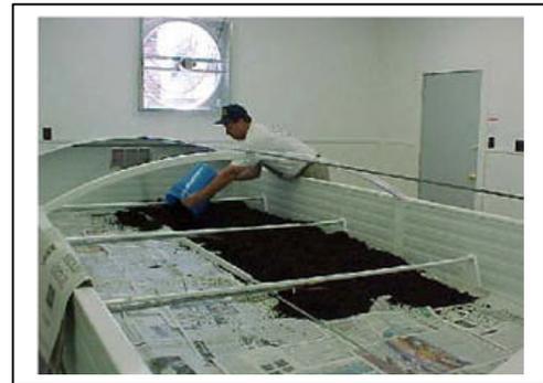
Feedstock is combined with cardboard, shredded and spread onto the surface of the bedding. Every 2 or 4 weeks the hydraulic system removes the bottom layer of castings, which are used by the grounds department. The system has a payback time of three years.
