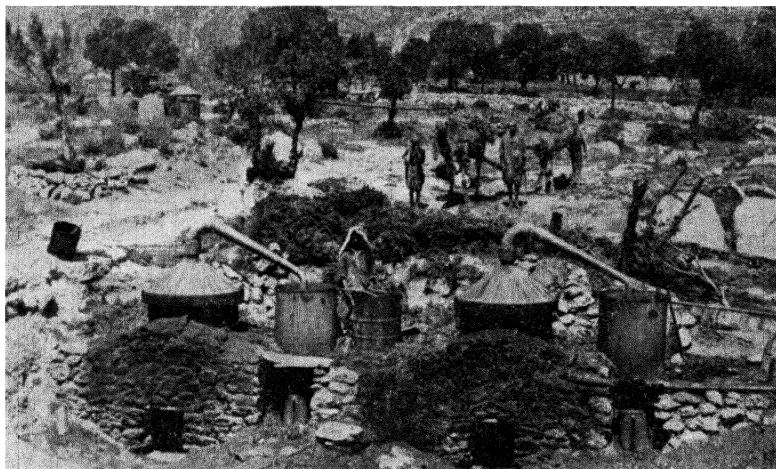
PLATE 4. Field distillation of rosemary in Tunis. The stills are directly fired. The plant material is transported by camels to the distillation post.
