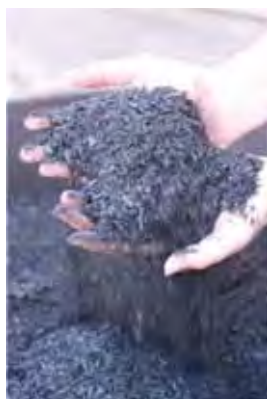
Figure 1: Biochar produced from a modern slow pyrolysis plant, operated by PacPyro, from greenwaste as a soil amendment and means to sequester carbon over the long term.
